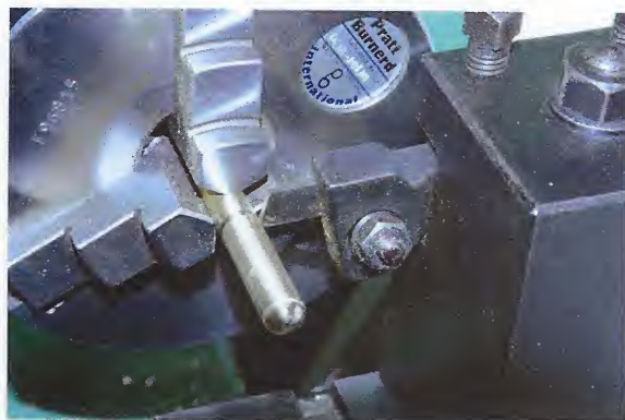
Fig. 56. Parting The Post
