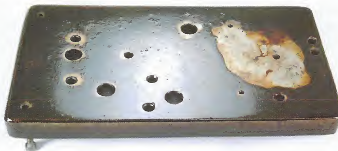
Fig. 12. Temp Too High Too Quickly
