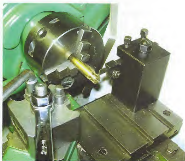
Fig. 2. Parting The Collet
