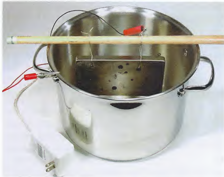
Fig. 10. Rust Removal From The Base
