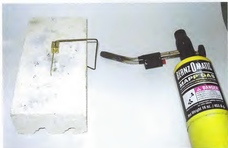
Fig. 47. The Rig For Brazing & The Torch
