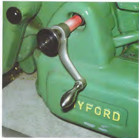
Fig. 37. The Crank Installed
