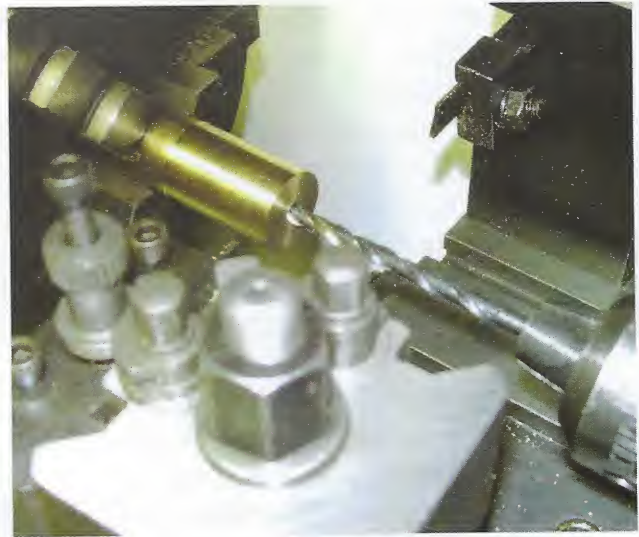
Fig. 10. Drilling The Weight Hole
