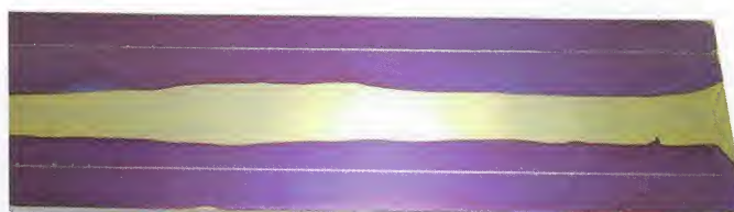
Fig. 17. Laying Out The Strip Conductors
