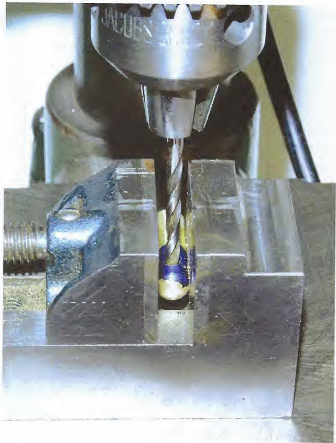
Fig. 60. Cross Drilling The Post
