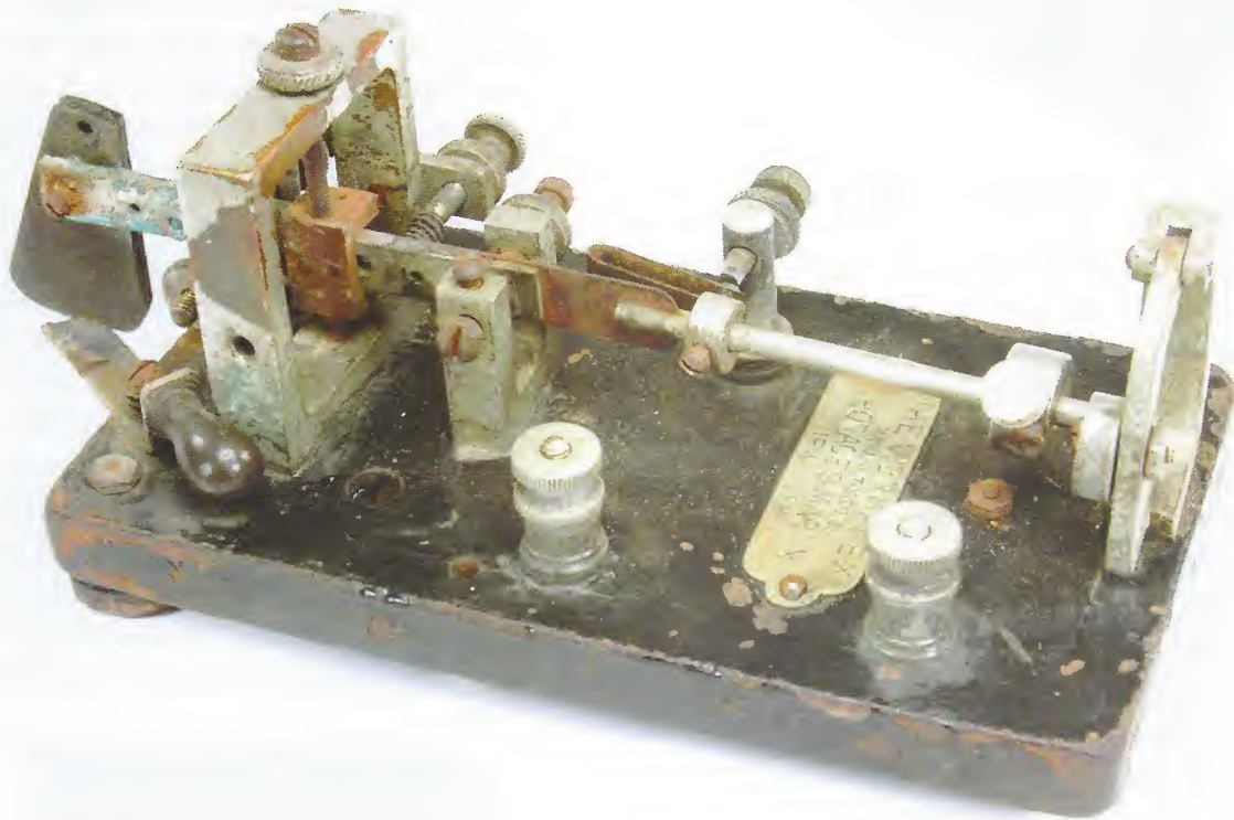
Fig. 1. A Double Lever Vibroplex Someone Converted To A Normal Key
