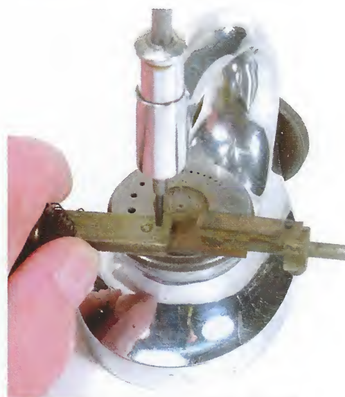
Fig. 86. Driving The Rivet From The Dot Bar
